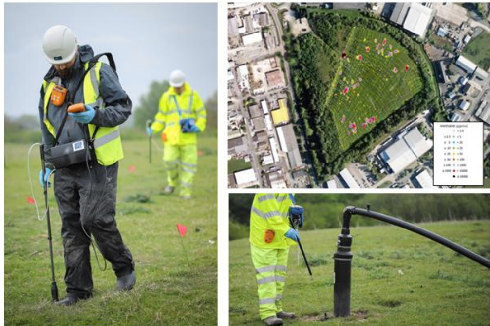
An example of a surface emission survey being carried out, and the resulting data.
