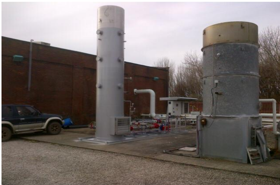
The prototype flare (on the left) at one of our UK demonstration sites.
