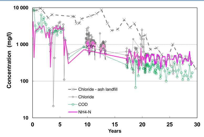
Leachate dilution at full scale landfills with high water inputs (Beaven et al., 2014)
